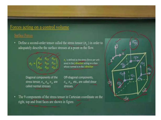
Now, if you come back to the surface forces, like for example, for tetrahedral structures like this where you have dx, dy, and dz components are there, and your axis is like this, x direction, y direction, and z direction. So, you can define the surface forces as a stress tensor. Stress means what, force per unit area. So, you can define as a stress tensor. So, this stress will have nine components. You could have this knowledge in solid mechanics.
