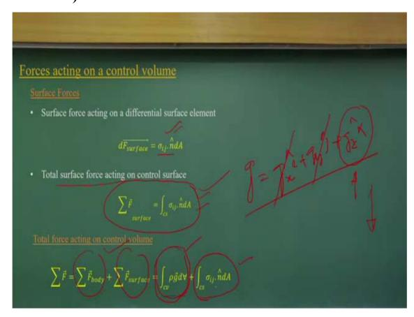
Surface force acting on a differential surface element
