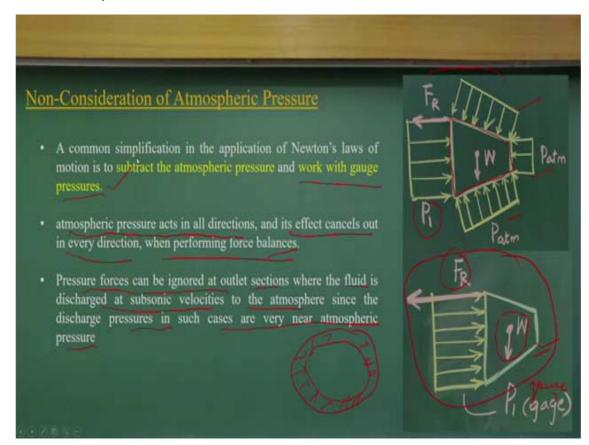
Now, let us consider very important component before applying this linear momentum equations. When you apply a linear momentum equations to a control volume, like I have the control surface like this, if you look at this control surface, in these three phases we have the pressure is atmospheric pressure. Here I have the absolute pressure, that means atmospheric pressure plus the gauge pressure.
