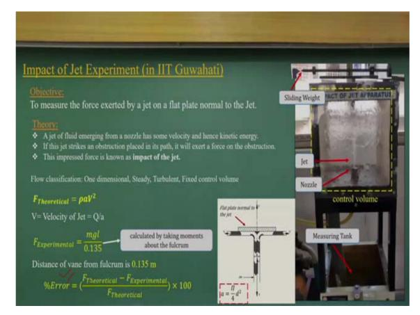
Now, before concluding today's lecture, let us see the figures, what is there, very simple experiment is impact of jet experiment. If you look at this jet, the water jet part is here and it is balanced by the weight here. So, we can know what is the velocity of impact if happening and that is how much of weight we are counterbalancing it. So, if you know it, theoretically, you know this is the control volume, you have water jet coming in and that water jet is going in these two directions.
